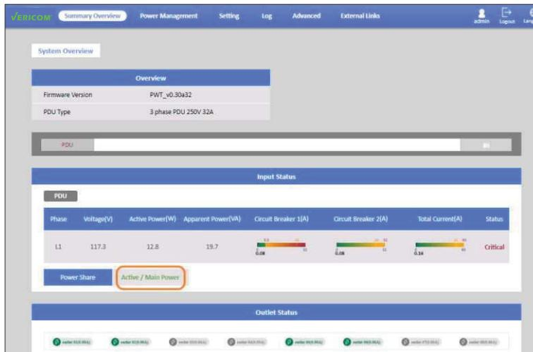
**Step 9:** The related log and trap will be recorded on the **Log** of the **Event Log** webpage and NMS. The log and trap will be “Information: Inlet (PDU:1) Active/Backup Power change to Active/Main Power”.
