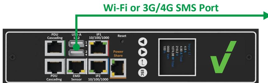
**Step 2:** Configure the related Wi-Fi or 3G/4G parameters on the **Wi-Fi Setting** of **Advanced** webpage. For example, to enable Wi-Fi Control, enter Wi-Fi SSI: TOTOLINK\_A1004...etc.
