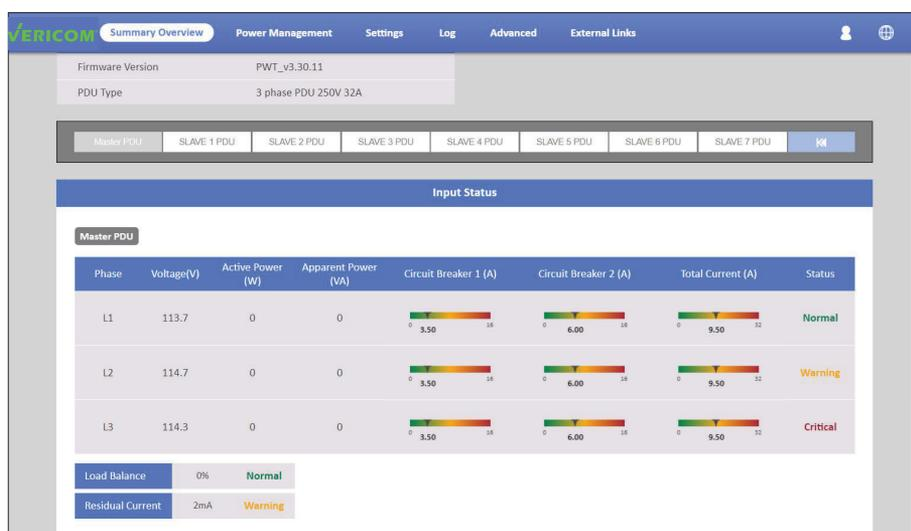
The main page shows a graphical representation of the PDU outlets and inputs status as described below:
