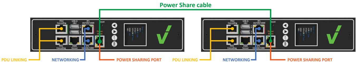
**Step 2:** After connecting the patch cable, open a web browser from a PC. The status of the power share is automatically displayed on the **System Overview** webpage. If PDU A is master PDU then the status of power share will display **Active/Main Power** on the **System Overview** webpage.
