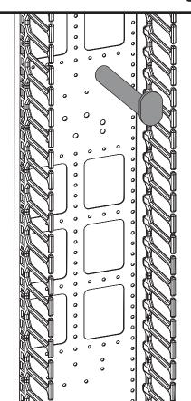
1. Locate any of the 6 pairs of 6mm dia. holes as shown.
